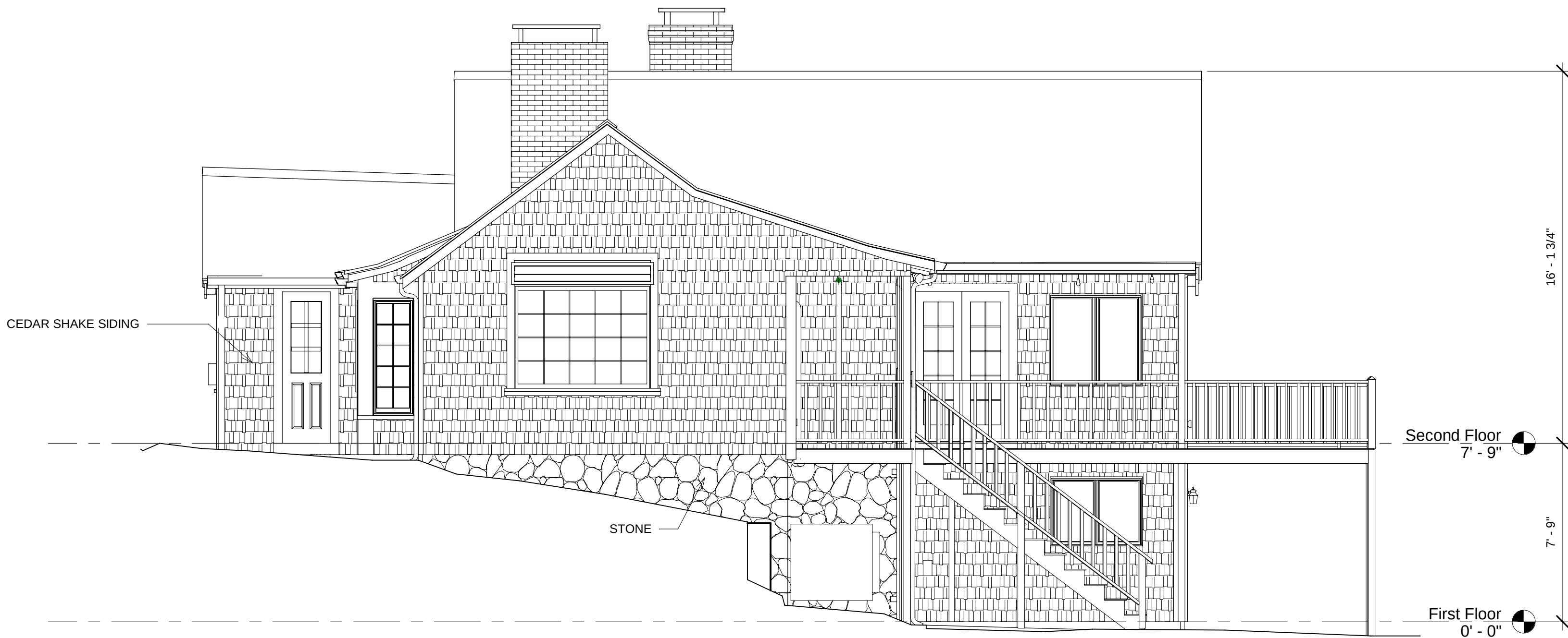
2 Existing North Exterior Elevation 1/4" = 1'-0"
